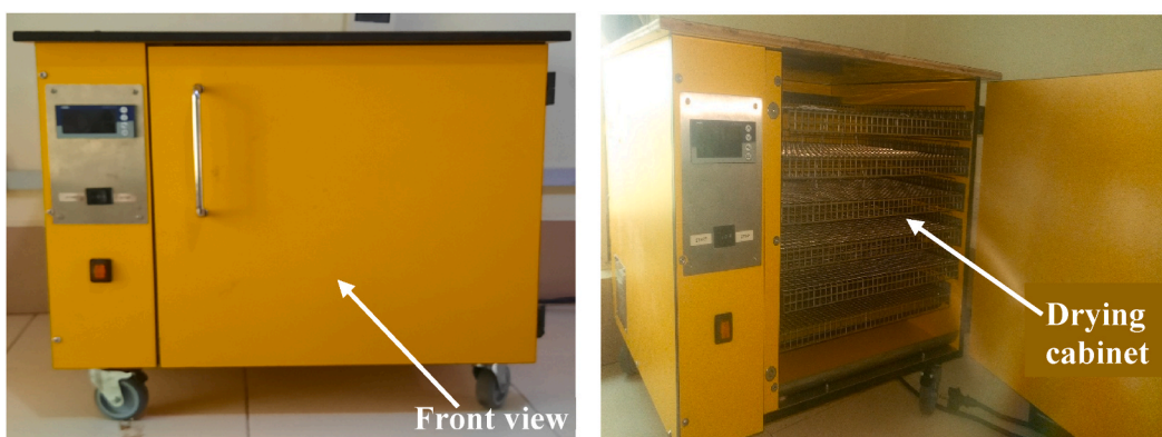
Fig. 1. Pictorial view of the bench top cabinet dryer.
