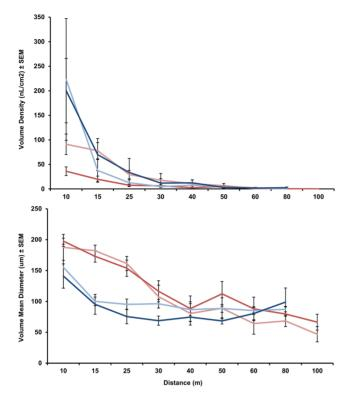
Figure 2. Volume density and droplet sizes of VectoBac WDG applied with a CSM2 and LV-8 at 400 and 800 g/ha in an openfield. Red = CSM2, blue = LV-8, light colors = 400 g/ha, dark colors = 800 g/ha. doi:10.1371/journal.pone.0110035.g002
