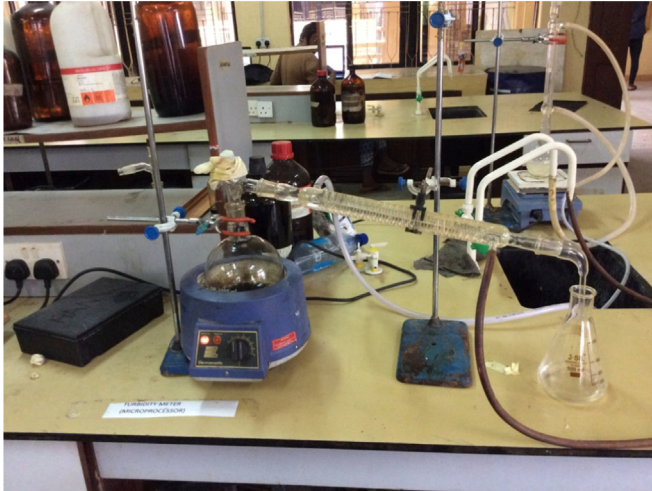
Fig. 1. Atmospheric distillation of oil for dehydration.
