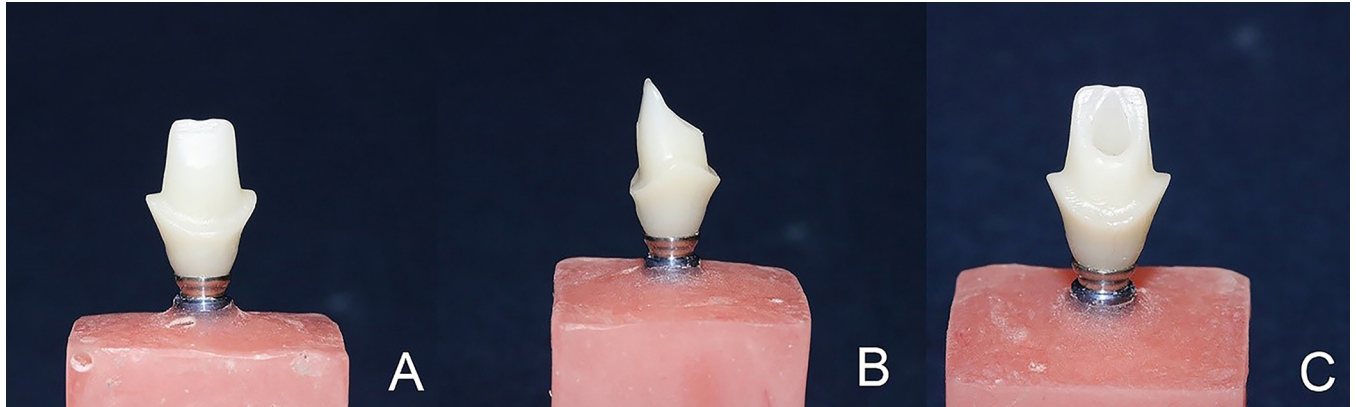
Fig 1. Milled customized zirconia abutment superstructure. A: buccal surface, B: proximal surface, C: lingual surface. The bonding surface of the titanium implant insert (ZrGEN; AnyOne; model: AAOIPR4525; Megagen, South Korea) was abraded with 50- \mu m aluminum oxide particles at a 10-mm distance for 10 seconds (0.4 MPa). The inner surface of zirconia abutment superstructures was also subjected to airborne particle abrasion with 30- \mu m silica-coated aluminum oxide (Rocatec Soft; 3M ESPE, USA).
