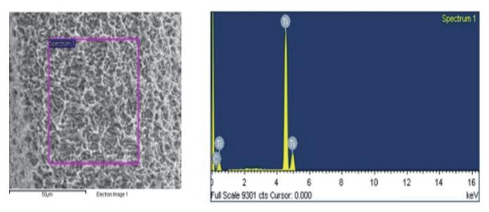
Fig. 5. Control group implant EDS spectrum. Ti and O were observed in SLA-treated implant surfaces.
