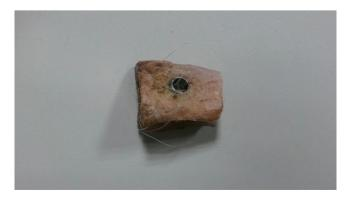
Fig. 2. Tibia sample including the inserted implant.
