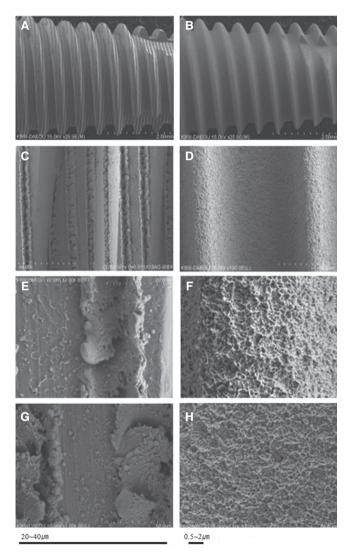
**Fig. 3.** Experimental and control group implant images obtained by field emission SEM: (A) Experimental group (×25); (B) control group (×25); (C) experimental group (×150); (D) control group (×150); (E) experimental group (×1,000); (F) control group (×1,000); (G) experimental group (×1,000); (H) control group (×1,000).
