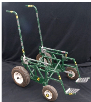
Figure 12. Surrogate wheelchair frame.
