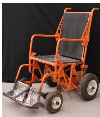
Figure 10. Surrogate wheelchair fixture.
