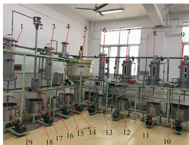
FIGURE 3 Sugarcane juice clarification experimental platform (1, 3, 6—heaters; 2—sulfitor; 4—diffusion box; 5—sedimentation tank; 7, 8, 9—evaporators; 10—syrup tank; 11, 12—equal pressure tanks; 13—evaporating hot water tank; 14—clear juice tank; 15—flocculant tank; 16—lime milk tank; 17—neutralizer; 18—neutralizing juice tank; and 19—mixed juice tank)
