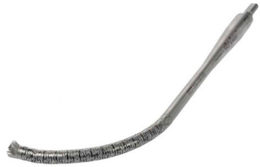
Figure 1. Flexible reamer with jigsaw design used to ream anatomic femoral tunnel through anteromedial portal.
