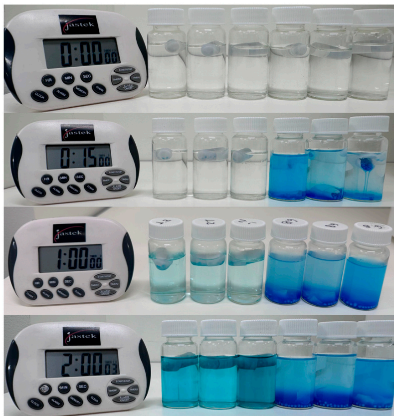
Figure 11. Time-dependent assessment of capsule integrity in different media. The three flasks on the left contain capsules in a pH 1.2 solution, and the three flasks on the right contain capsules in MilliQ water (pH 5.1). The image captures the state of the capsules at 0 h, 15 min, 1 h, and 2 h, highlighting the delayed disintegration in acidic conditions compared to the rapid release at pH 5.1.
