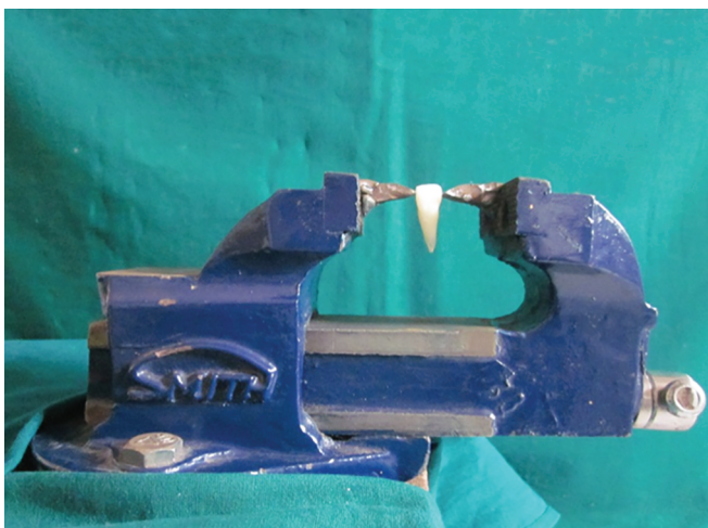
Fig. 1: Custom-made blade mounted on a vise to induce Ellis class II fracture
