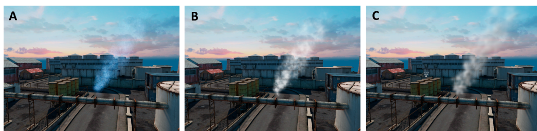
Figure 5. The same gas plume, as visualized with each of the presented methods: (A) billboarded 2D assets, (B) procedural textures from OpenSimplex noise, and (C) volumetric rendering through ray marching.
