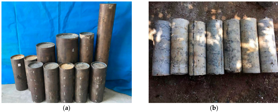
Figure 5. Typical failure mode of specimens. (a) Failure mode of all specimens; (b) The core concrete taken out from partial CFT-PAC columns.
