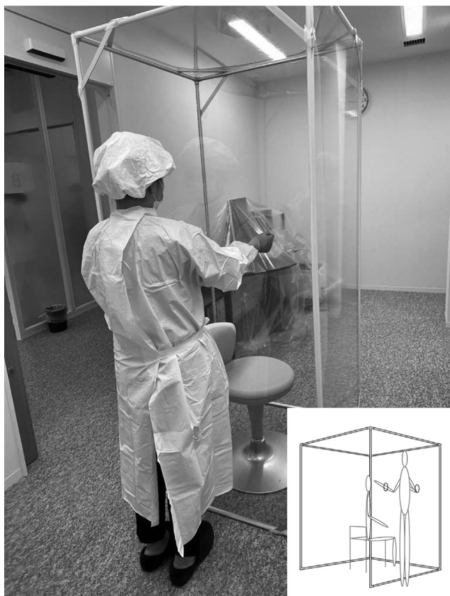
Figure 1. Protective barrier box. The box is 900 mm (width) × 2000 mm (height) × 900 mm (depth) in size, and is constructed using a steel frame and soft plastic. On one wall of the box, two arm holes allow access for sampling.
