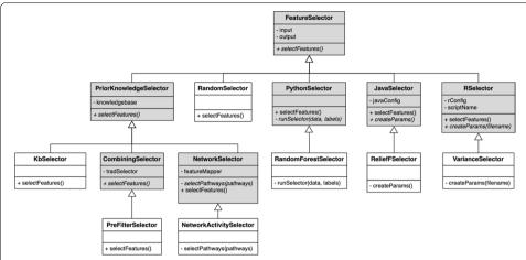
**Fig. 3** Class structure of the FeatureSelection component (abstract classes in grey). On top of the hierarchy is an abstract FeatureSelector class that defines the method selectFeatures(). This method is invoked during pipeline execution. Actual feature selection strategies are realized in inheriting classes
