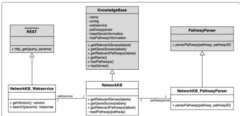
**Fig. 4** Example implementation of a knowledge base providing network information. Class *NetworkKB* inherits from the abstract *KnowledgeBases* class to implement the required interface functions. Class *NetworkKB\_Webservice* retrieves the actual prior knowledge from a web service via their REST APIs. As network information is retrieved, *NetworkKB\_PathwayParser* parses the network information and transforms it into a uniform format that is used by Comprior
