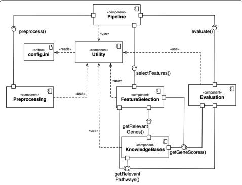
**Fig. 2** Overview of Comprior's system components. There is a major Pipeline component for benchmark orchestration, while specific functionality is implemented in dedicated components. Communication between the components is realized via corresponding interface methods
