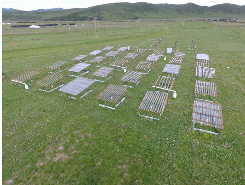
Figure 6. Plot layout and experimental design of the study. The varying levels of precipitation are achieved using combinations of water catchment and rainout shelters.
