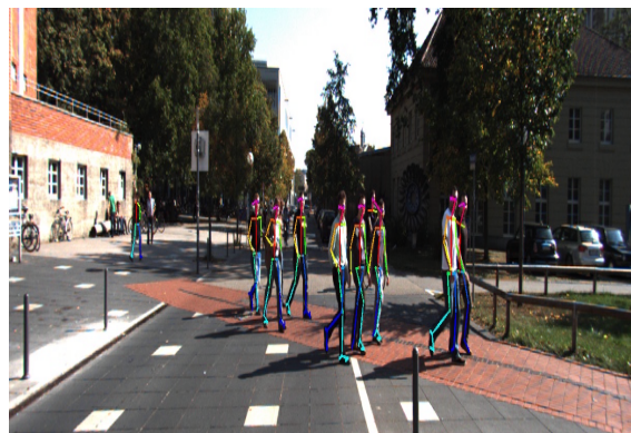
Figure 5. Result of OpenPose joints detection. The training sequences number 16 of the KITTI tracking benchmark.
