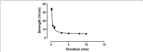
**Fig. 3** Defibrillation probability strength–duration curve.  $R^2 = 0.9885$  (Weiss–Lapicque equation). Points indicate the electric field associated with 50% of defibrillation success (HEF<sub>50</sub>) and the vertical lines indicate the confidence interval for 95%. Curve was fitted by Eq. (1) (rheobase =  $4.17 \pm 0.561$  V/cm, chronaxie =  $1.41 \pm 0.235$  ms), n = 10, each heart was defibrillated seven times (one time for each pulse duration)
