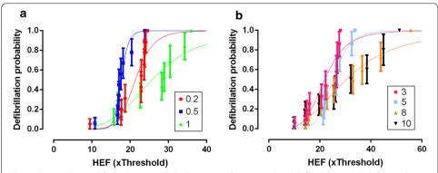
**Fig. 4** Curves obtained from the sigmoidal adjustment of the normalized defibrillation probability result as a function of the electric field ( $\times$ Threshold). Vertical lines indicate standard error of the mean (SEM). **a** Curves of the durations 0.2-, 0.5- and 1-ms. **b** Curves of durations 3-, 5-, 8- and 10-ms. Curves were fitted by Eq. (3), n = 10
