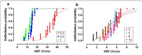
**Fig. 2** Defibrillation probability as a function of the applied electric fields (V/cm). Vertical lines indicate the standard error of the mean (SEM). **a** Curves of the durations 0.2-; 0.5- and 1-ms. **b** Curves of durations 3-, 5-, 8- and 10-ms. Curves were fitted by Eq. (3), n = 10, each heart was defibrillated seven times (one time for each pulse duration)
