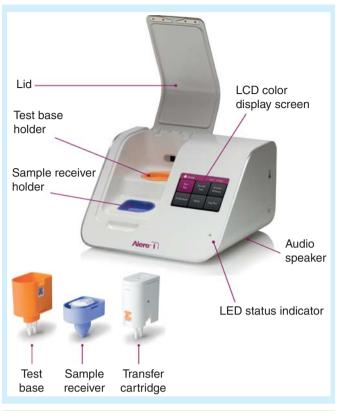
**Figure 2. The Alere i molecular diagnostics platform and sample processing components (inset).** Figures provided courtesy and permission of Knowledge Optimization<sup>®</sup>, Davis, California, and Visual Logistics.
