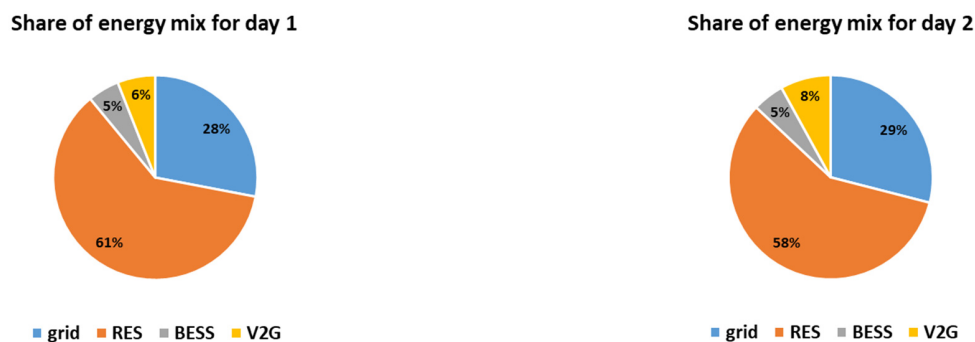
Figure 10. Share of the energy mix for the two simulated days considering the worst-case scenario for the RES production time-series forecast.
