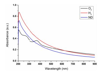
**Figure 2.** Absorbance spectra of oxygenated nanodiamond particles (ND 1), hydrogenated nanodiamond particles (ND 2), and unmodified nanodiamonds (ND 3).
