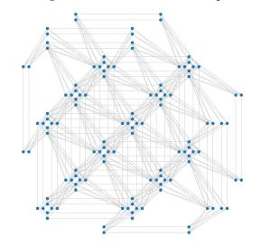
**Figure 1.** Portion of a Pegasus graph used in Advantage QPUs. Nodes represent qubits, while edges show the connections between qubits. The cross form of several Chimera cells is clearly visible.
