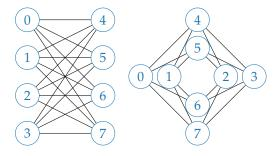
**Figure 2.** Chimera unit cell in its two common renderings, bipartite and cross form, with numbers representing qubits in the cell. We can see that each qubit is connected to 4 others of the same cell. Further connections, shown in Figure 3, connect different cells.
