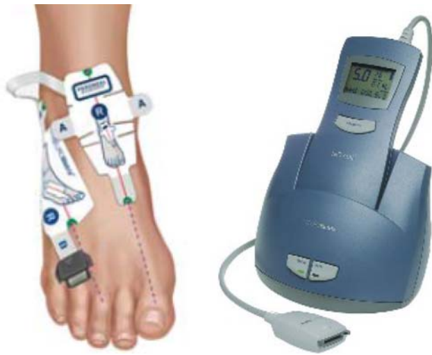
Fig. 1. Photograph of the NC-stat instrument. It consists of three components: pre-fabricated electrode arrays (biosensor, left panel) for a peroneal motor nerve conduction study, an electronic monitor (connected to a biosensor during testing), a report generation system (not shown) based on electrophysiological data collected and processed by the monitor and transmitted via “docking station” (a telecommunication port for secure data transfer via telephone line).
