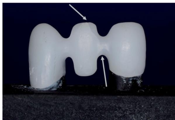
**Figure 1.** Fracture of a non-colored FDP framework propagating from the mesial side of the connector to the site of the indenter. Fracture marked by arrows.
