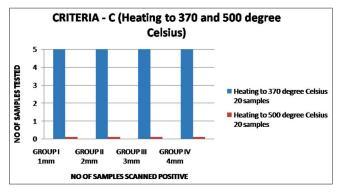
Figure 10: Graph demonstrating result when QR codes were heated drastically (Criterion C)
