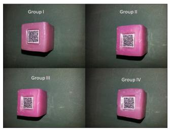
Figure 2: QR code incorporated in samples of Group I, II, III, and IV
