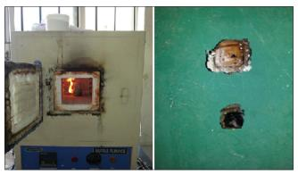
Figure 6: Sample burned at 500°C
