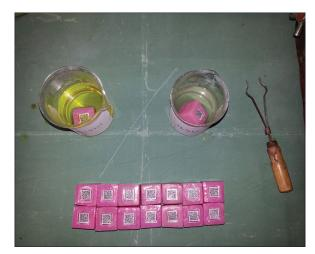
Figure 4: Samples treated with sulfuric acid (99%) and hydrochloric acid (40%)
