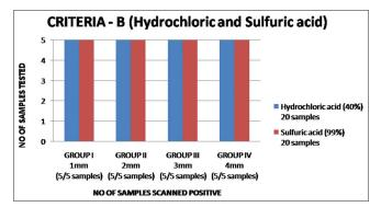
Figure 9: Graph demonstrating result when QR codes were exposed to inorganic acids (Criterion B)
