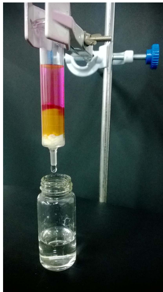
Figure 7 | Demonstration of drinking water purification by regenerated \text{SiO}_2 @PEI@AZ/PEG adsorbent. Red: Rhodamine B labelled water for better demonstration. Yellow: adsorbent. White: cotton (to prevent leakage of adsorbent).
