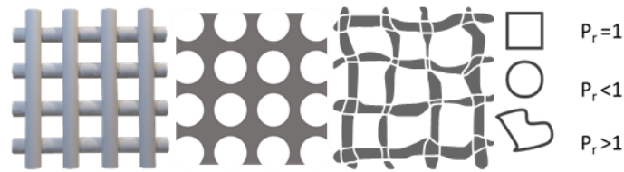
Figure 14. The influence of pore shape on the P_r index in a grid structure. The schematic structure was designed based on Ouyang et al. [35].
