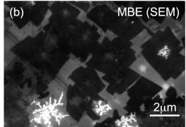
Figure 1. Distribution of graphene flakes in the CVD and MBE synthesised samples on Ge(001). Conductive graphene is dark in SEM images for (a) CVD and (b) MBE grown graphene.
