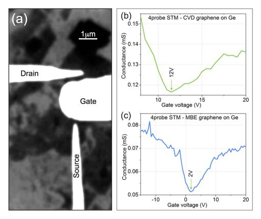
**Figure 4. Electrical measurements with 4-tip STM.** (a) SEM image of the tip arrangement in the FET configuration. One tip serves as a transistor gate and two other act as the source and drain contacts. (b) Graphene channel conductance as a function of the gate voltage: a CVD sample, tip-sample distance d = 15 nm. (c) The same for an MBE sample, d = 25 nm; the graphene is here separated from Ge(001) by a graphene-like interfacial layer<sup>23</sup>.
