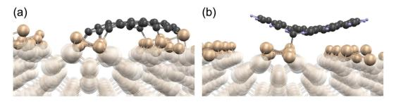
Figure 6. Small graphene molecule (29 atoms) on Ge(001)- $p(2 \times 2)$ . (a) MBE: the edge C atoms tend to make bonds with the substrate. (b) CVD: the edge C atoms are terminated with H, and some of these atoms (here: one atom) makes a weak bond to the substrate.
