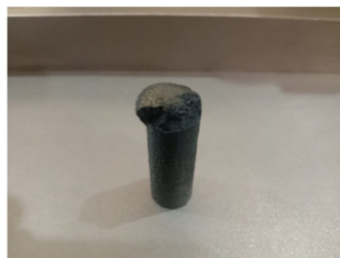
Figure 5. Chipping of specimen under loading condition: above 100 N.
