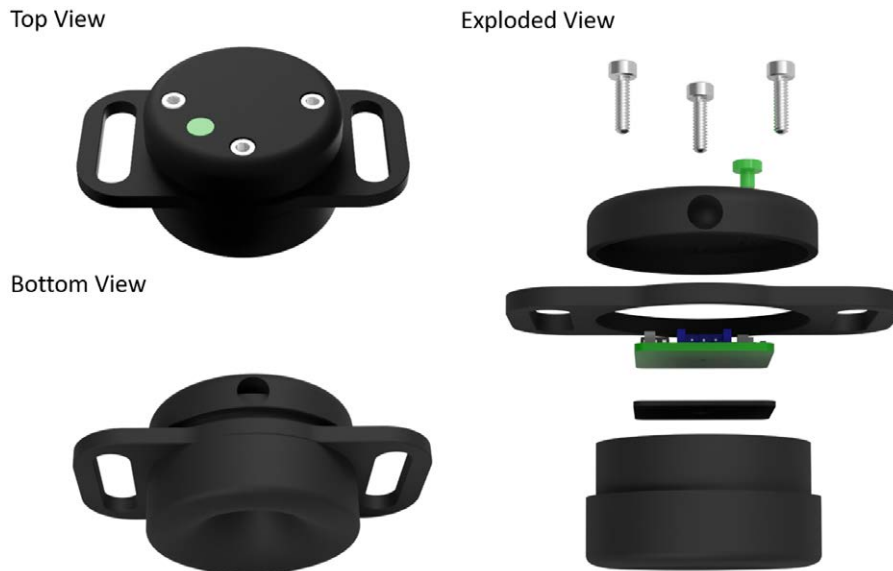
Fig. 1. Renderings of the surface microphone. Green elements represent the circuit board and the led “on light” indicator.
