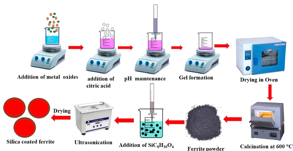
Figure 1. Illustration of synthesis and silica coating of \text{Cu}_{0.50}\text{Mg}_{0.50}\text{Fe}_2\text{O}_4 adsorbent.
