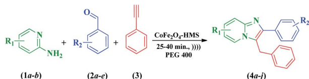
Scheme 1 Synthesis of imidazo[1,2- a ]pyridine derivatives ( 4a–j ).
