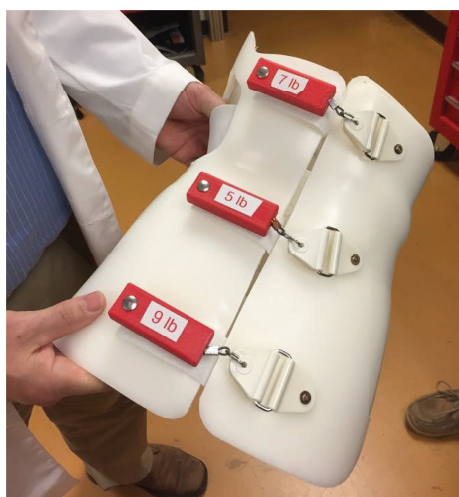
FIGURE 3: CTU devices mounted on a conventional brace in-line with the posterior fastening straps.
