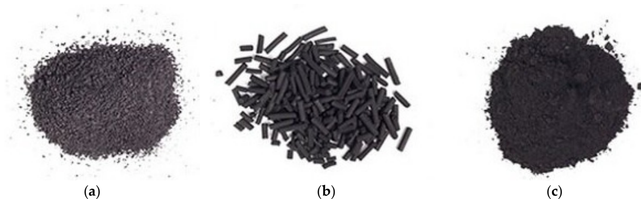
Figure 3. Representation of (a) granular, (b) pelletized and (c) powdered types of activated carbons. Reprinted with permission from Ref. [92].
