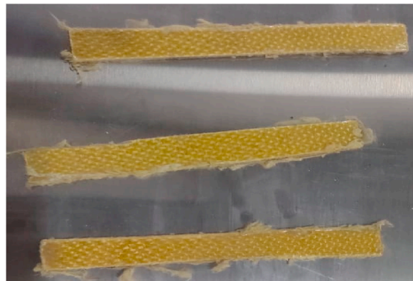
Fig. 5. Impact strength of composite test sample.
