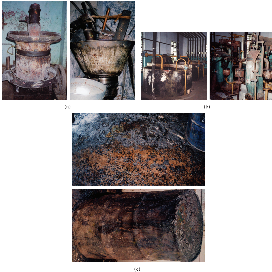
FIGURE 2: Oil production and spillage. (a) Crushing system in small-scale oil production. (b) Crushing system in large-scale oil production. (c) Spillage from oil production points. These releasing points are potential sources of environmental issues.
