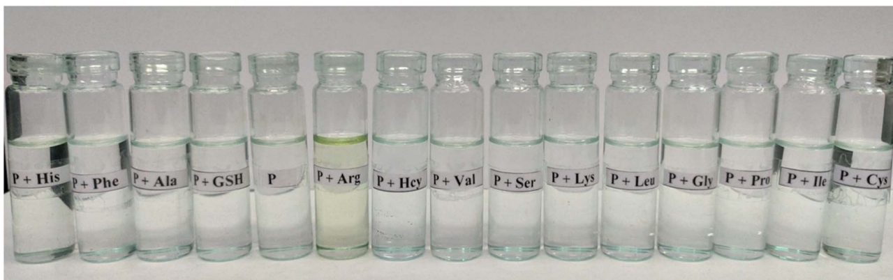
Fig. 1 Colorimetric variations in PPS (10 \mu\text{M} ) on addition of 10 equiv. of different amino acids.
