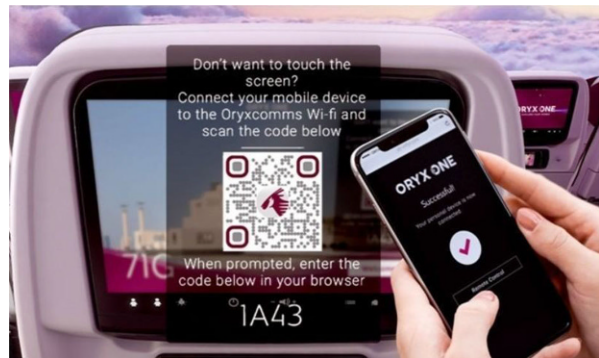
Fig. 5 Screen takeover via QR code on Qatar Airlines to use the seat-back smart screen without touching [17]
