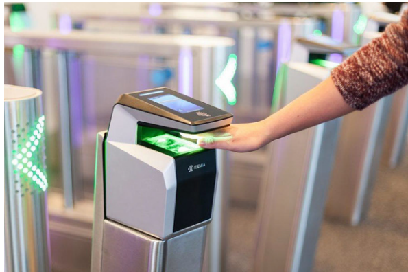
Fig. 1 Touchless biometric fingerprint access control for entrance gate [8]
