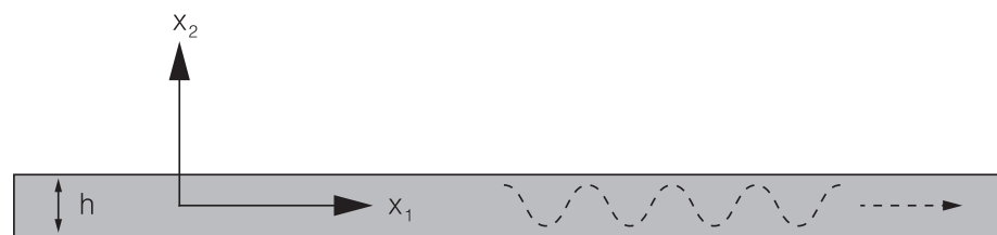
Figure 3. Geometry of the waveguide.
