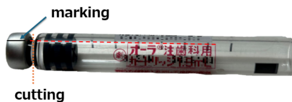
Fig. 3. Marking and cutting positions in cartridges. The marking positions were set by referring to the cartridge labels to capture photographs that overlapped the 20 cartridges. After the marking, the neck of the cartridge was removed.
