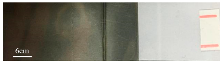
Figure 4. The joining sample of oxygen plasma-treated PS and laser-oxidized titanium.
