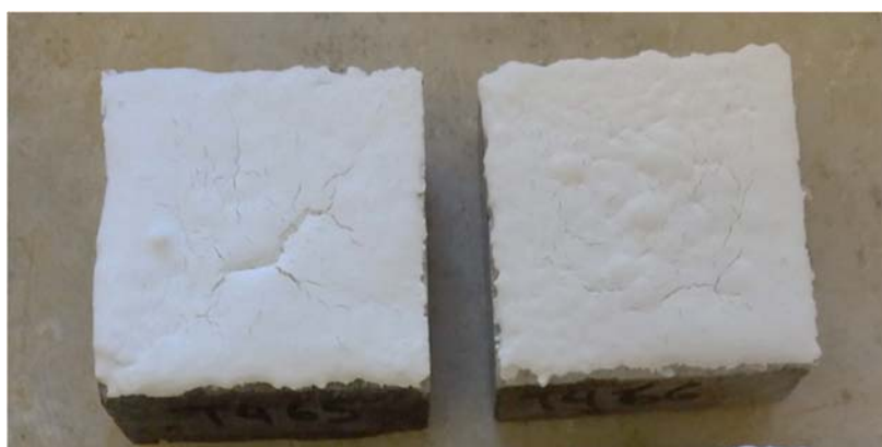
Figure 4. Concrete blocks (specimens) coated on one side (50 × 50 mm) by the M1cm sample.
