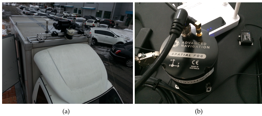
Figure 7. Sensors for the test on the ground. GPS is used to calculate the velocity of the vehicle. (a) Sensors on the roof of the test vehicle; (b) Fiber optic gyroscope (FOG) and attitude heading and reference system (AHRS) inside the vehicle.
