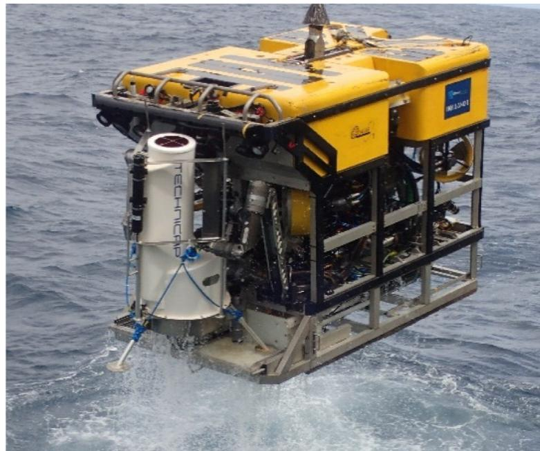
**Figure 2.** The Holland I ROV recovering a Little MonSta after successful deployment. Note the ROV 7 function manipulator arms clamping the lander to the ROV whilst resting on the ROV chassis. As a fail-safe, the lander is also hooked to the ROV.
