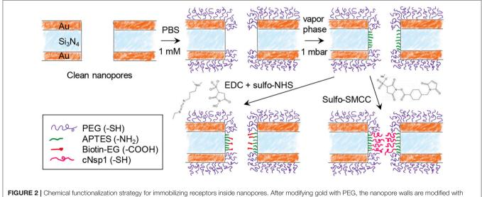
FIGURE 2 Chemical functionalization strategy for immobilizing receptors inside nanopores. After modifying gold with PEG, the nanopore walls are modified with APTES. Receptors can then be bound by cross-linking chemistry between -NH<sub>2</sub> and -COOH (EDC + sulfo-NHS) or between -NH<sub>2</sub> and -SH (sulfo-SMCC). Using sulfo-SMCC is more challenging as it requires that the thiol-PEG coating prevents other thiol groups from reaching the gold.
