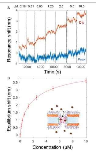
**FIGURE 4 | (A)** Detection and titration of Kap $\beta$ 1 binding to smaller pores modified with cNsp1. Kap $\beta$ 1 is introduced at increasing concentrations and the equilibrium signal is obtained by averaging over time (at least 10 min for each concentration, corresponding to ~1,000 values). **(B)** The equilibrium signal for the different concentrations introduced. The curve shows a fit to the two component Langmuir model.
