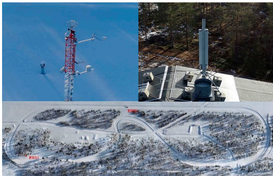
Figure 3. Test-track equipped with the 5G Test Network (5GTN) base station and Road Weather Stations (RWSs).
