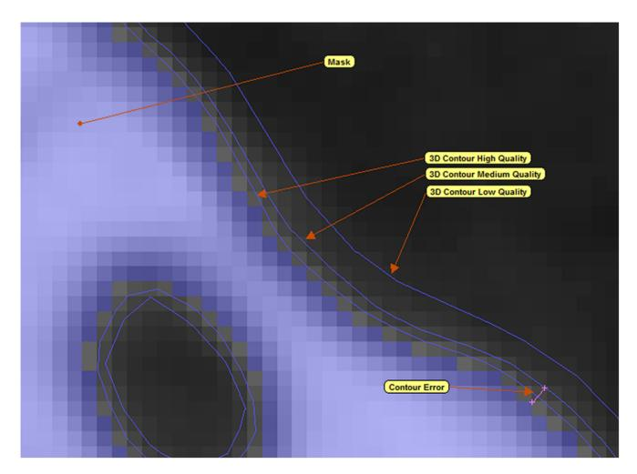
**Figure 7. Quality of isosurface models and error quantification.** The mask (shown in blue) represents the segmented/selected voxels that will be used to create isosurfaces. The three different contour qualities represent the 3D approximation of the mask and will form the isosurface. Contour error is the measured distance between the isosurface contour and the mask it was generated from (lower left of image). doi:10.1371/journal.pone.0053873.g007
