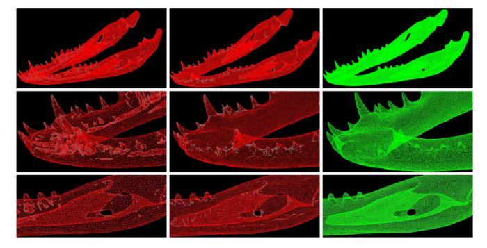
**Figure 8. Mesh optimisation and solid mesh generation.** Mesh optimisation and solid mesh generation was performed using Harpoon (SHARC). The left images show the complex internal geometry captured from isosurface generation. The middle column shows removal of complex internal geometry whilst still retaining important geometrical features. Images at right show the final solid mesh. doi:10.1371/journal.pone.0053873.g008
