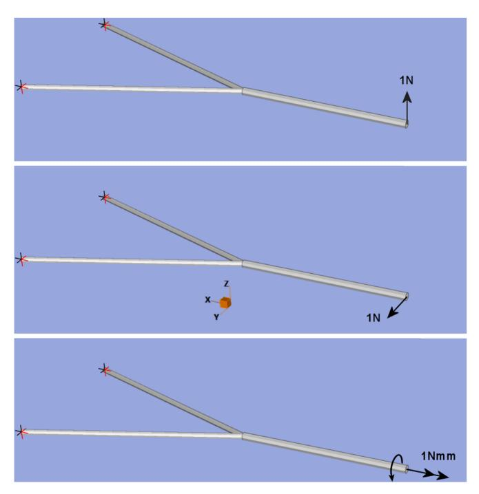
**Figure 11. Beam models showing axes, restraints and loads.** From top; shows loads and restraints for *biting, shaking* and *twisting* respectively. In all three cases models are fully restrained (rotation and translation) at the most posterior points of the beam model. Loads are all placed at the most anterior point of the beam model. doi:10.1371/journal.pone.0053873.g011
