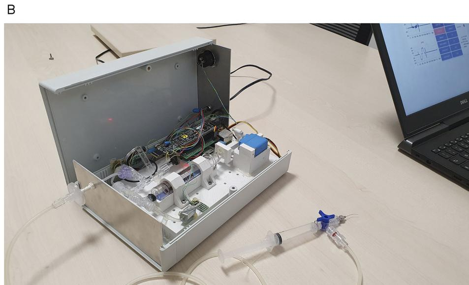
**Figure 1.** Schematic of the components of the device (A). Prototype used for the study experiments (B). box open to show components.
