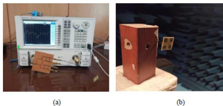
Fig. 20. Measurement setup, (a) antenna connected to the network analyzer, and (b) antenna placed in an anechoic chamber.
