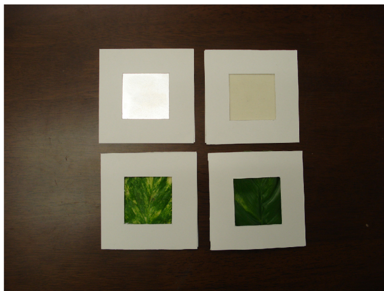
Figure 1 Tactile samples. The samples are, clockwise from top left, metal, fabric, artificial pothos, natural pothos.
