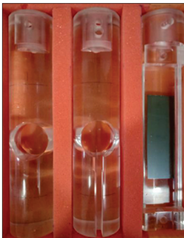
Figure 4: Cylindrical polymethylmethacrylate inserts for the target, ionization chamber, and radiochromic film samples, respectively (left to right)
