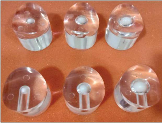
Figure 2: Polymethylmethacrylate inserts with Delrin® target of diameters 1.0, 1.5, and 2.0 cm from left to right (top row). Bottom row shows inserts of the same diameter as above, along with the cavity for placing different dosimeters
