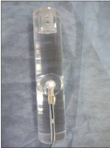
Figure 3: CC13 ionization chamber placed into the polymethylmethacrylate dosimetry insert
